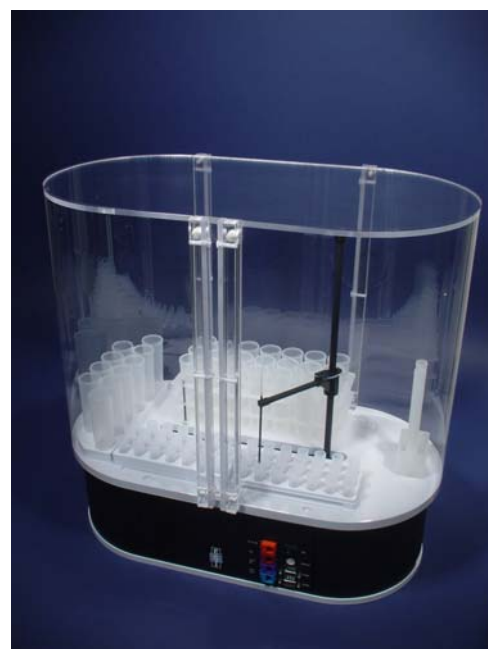
SC-2 autosampler with clean enclosure attached
