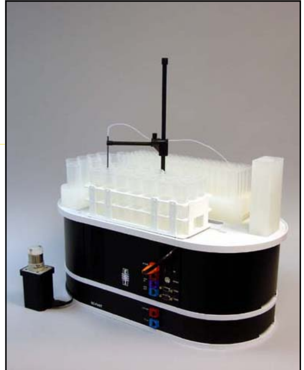
The FAST system integrated to the SC-2 autosampler includes control of an inert injection valve for sample injection or chromatography applications.
