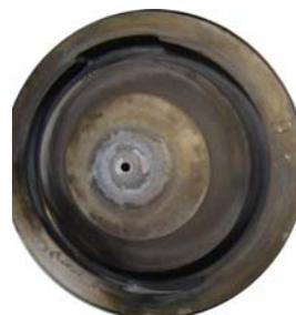
Salt free ELAN sampler cone after >300 GSL samples
