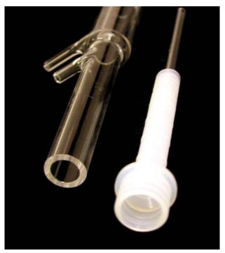
The precision quartz torch and o-ring free injector directly replace the standard Leeman demountable torch and injector.
